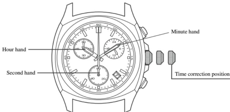
In the case the crown is of the screw-lock type, loosen the screw by turning the crown to the left before operating the crown, and after having returned the crown to the normal position following operation, turn the crown to the right while pushing it in to securely retighten it.
