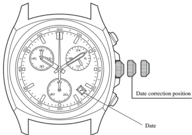
1. Pull the crown out to the date correction position.
